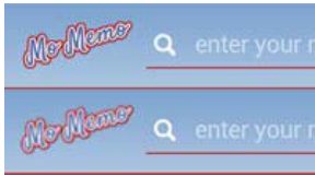
Figure 6-3. High-resolution images (bottom) vs low resolution (top) on a high density display
